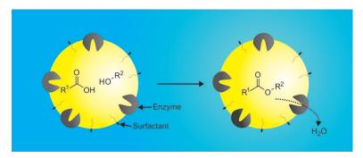
Just a drop of water: Esterification in water is possible by confining the reactants in small miniemulsion droplets protected by nonionic surfactants. A lipase located at the interface between the droplet and aqueous surroundings
