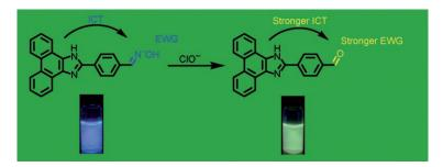
The first ratiometric fluorescent probe for hypochlorite has been developed through regulation of the electronwithdrawing ability of the electron acceptor in an intramolecular chargetransfer (ICT) system by a deoximation reaction (see figure; EWG = electron-withdrawing group).
