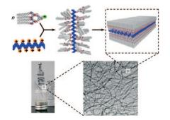
Let's stick together: The gelation ability of a dendritic gelator has been enhanced by its complexation with a polyelectrolyte (see figure). This concept provides a route to construct novel functional or ordered materials by complexation of other low-molecular-mass functional species with polyelectrolytes.
