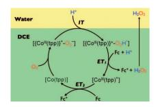
Oxygen reduction: A polarized water |1,2-dichloroethane (DCE) interface acts as a proton pump for the [Co-(tpp)] (TPP=5,10,15,20-tetraphenyl-porphyrinato) catalyzed  $O_2$  reduction by ferrocene (Fc) compounds to produce  $H_2O_2$  (see figure; IT=ion transfer, ET=electron transfer). This system favours the collection of  $H_2O_2$  by extraction immediately after its formation in DCE to the adjacent water phase.
